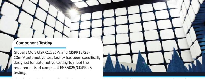
The chamber is also compliant for immunity tests to ISO 11452-2 and is constructed using a self-standing steel structure and modular steel shield.
