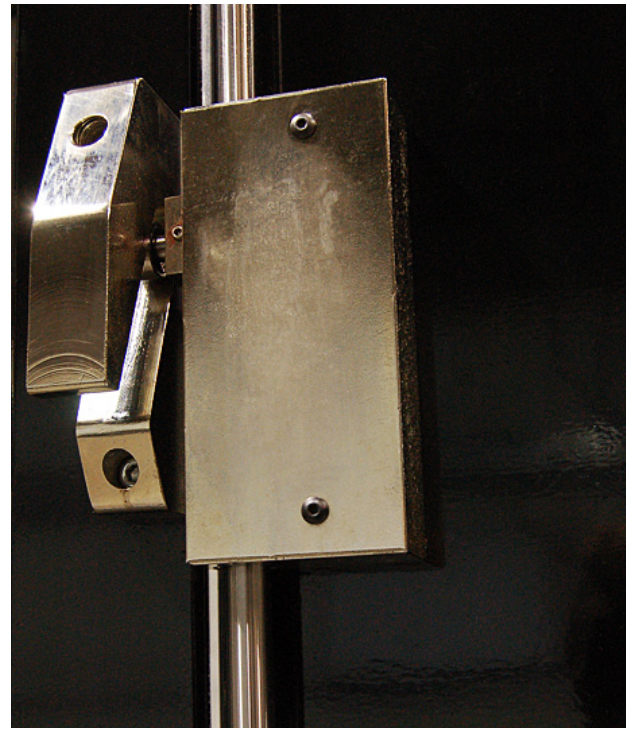
All interfaces have roller bearings for easy open/close operations
